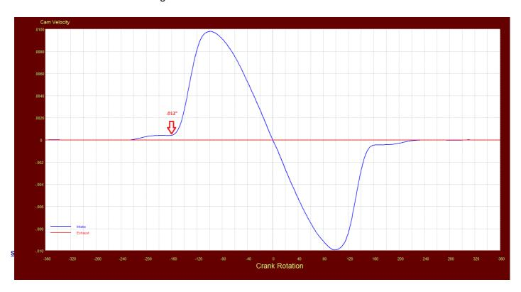
In our DOHC example shown above, the first two pictures show correct clearance at .012" and what the valve train is seeing on the velocity curve. the following two pictures show when the lash is set . 004" looser than recommended and how it looks for the poor valve train on the velocity curve.
