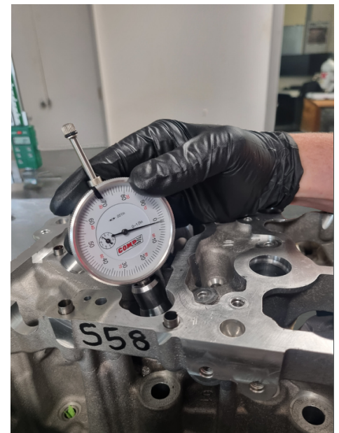
Figure 6 : Measuring Valve Tip Height in the S58 head
