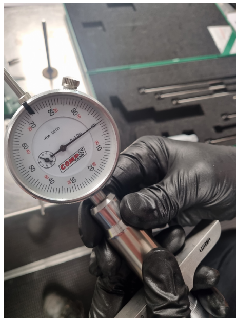
Figure 5 : Calibrating Dial Gauge for Valve Tip Height Measurement
