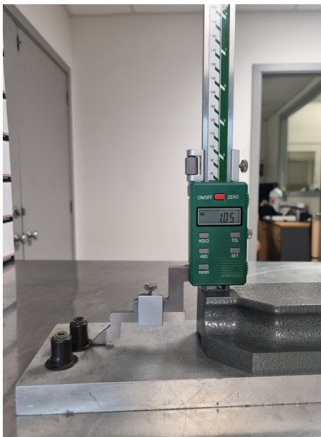
Figure 4 : Confirming Spring Base Stem Seal Thickness
