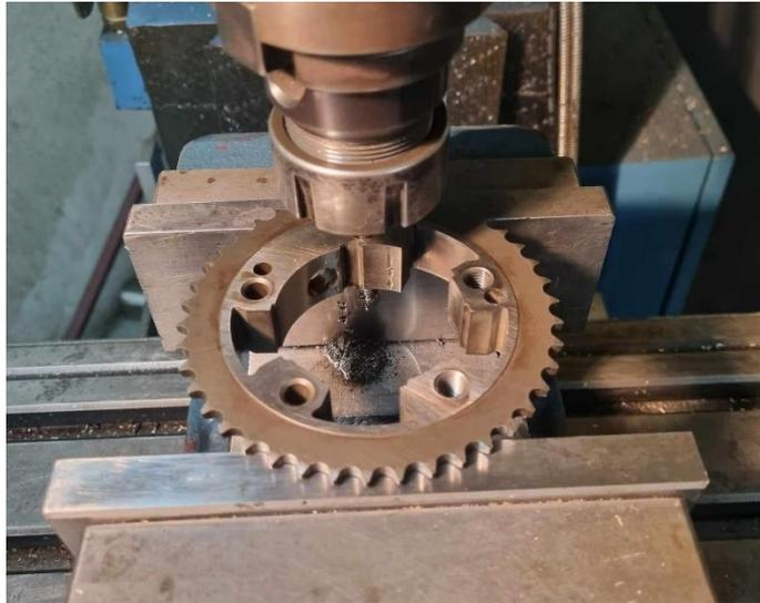
4. Tap the old bolt holes with the M8\*1.25 Tap, there will be 5 bolt holes on each gear that require aligning and tapping. The cam gears are made from a very hard material so will need to be tapped slowly with plenty of fluid.
