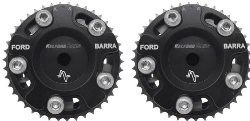
8. The Kelford Cam gears are designed to be installed at the full retarded position. This is to account for Race engines which have had the heads/blocks surfaced which will affect the cam timing. These need to be timed up and dialled in as per the Kelford Cam Timing instructions found on our website.
