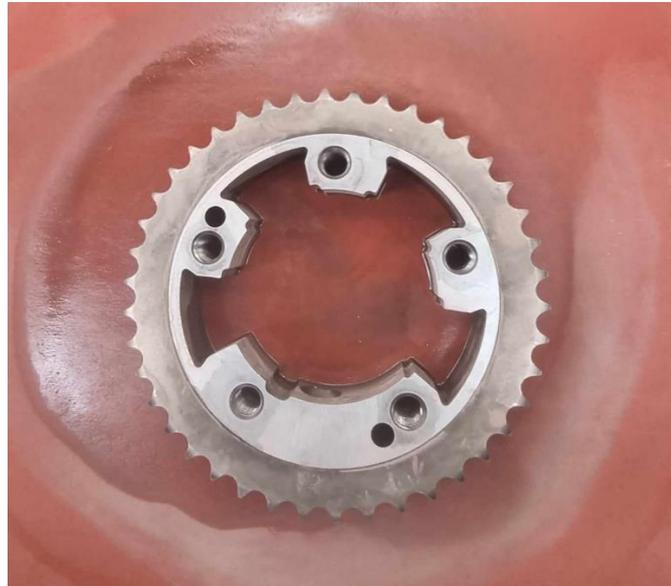
6. Remove the Kelford Cams KCGBARRA gear inserts from the packaging along with the 10 x M8\*1.25 stainless cap screws.
