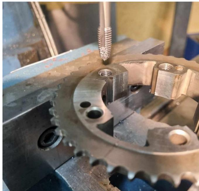
5. Gently lap the cam gear faces with wet 600 grit on a flat surface to remove all burrs. Thoroughly clean the gears so they are ready for assembly.
