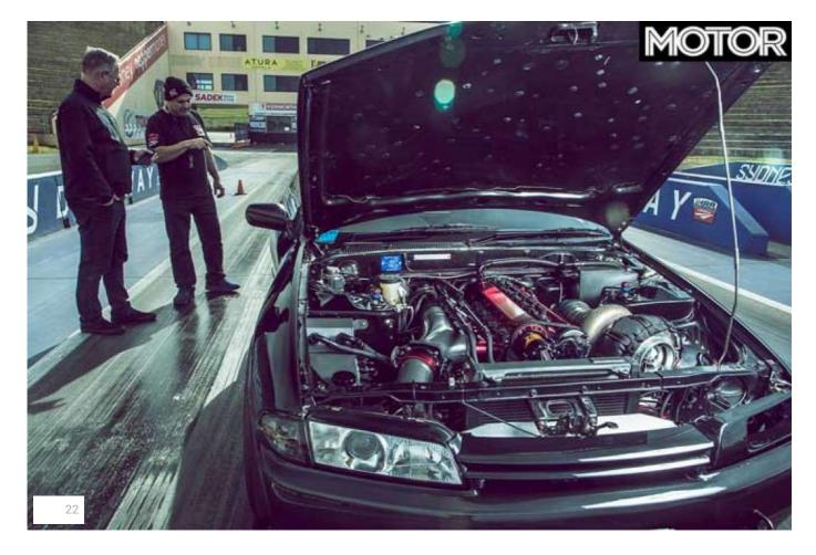
Under the steel bonnet lies a Nitto-stroked 3.2-litre RB30 with a billet block, fed United E85 by 12 fuel injectors and a customised under-bonnet surge tank on the right guard. The Precision XP098 turbo could hide a rockmelon, and can handle up to 2300bhp, according to Rob, while the whole shooting match is orchestrated by MoTeC.
